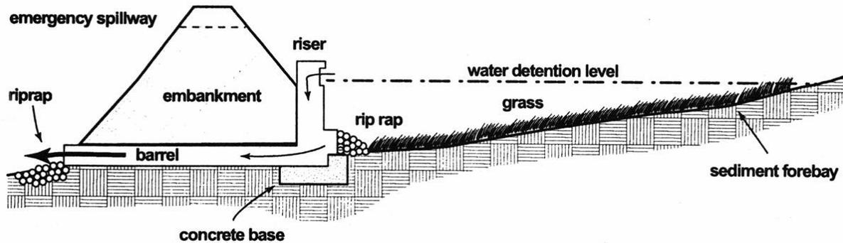
Figure 2: Typical Dry Detention Basin Section
